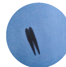
TWO THICK LINES SHOW WHEN CARTRIDGE IS CLEANED
